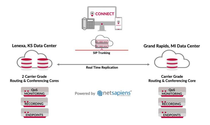
The unique geo-redundancy technology allows all modules to act as one single switch when distributed across different locations. All call state information, all feature codes, all voicemail is replicated in real-time to all the other servers. In addition, phone devices are configured for SRV, allowing for registration to multiple servers.
